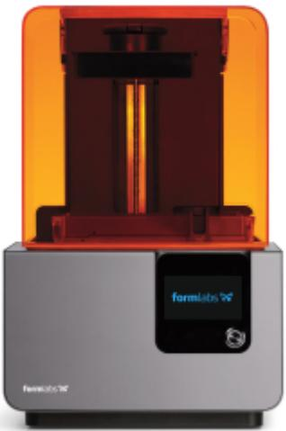
A photograph of a FormLabs Form 2/3 SLA 3D printer. The printer has a black base unit with a small digital display and a grey side panel. On top of the base is a clear acrylic build plate with a black frame, and above that is a translucent orange resin bath. The printer is shown from a front-three-quarter angle. |                               |
