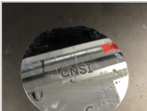
Contour cut in 0.5mm SI wafer
