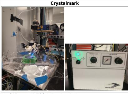
Tool Type: CNC Airjet Abrasion Cutter
