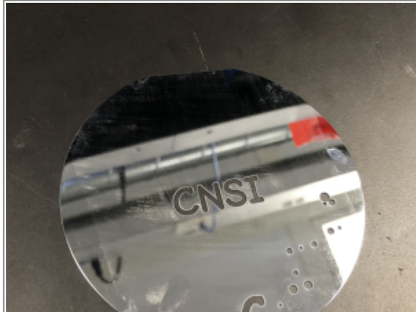
Contour cut in 0.5mm SI wafer
