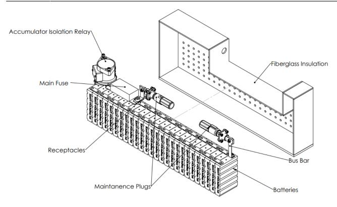
26s5p li-ion cells per segment comprised of Enepaq 1x5p Sony VTC6 modules
