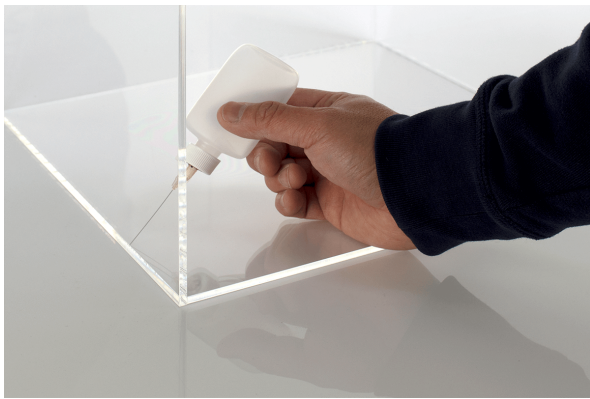
Fig. 2: Application of methylene chloride to joints via capillary action.
