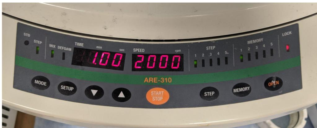
I) Operation Mode: The device can operate in standard (STD) and stepwise (STEP) modes. Stepwise mode allows access to multiple steps of operation and enables the user to vary the revolution speed, while standard mode only allows for variation of mixing time within one step. You can switch between these modes using the **MODE** button.
