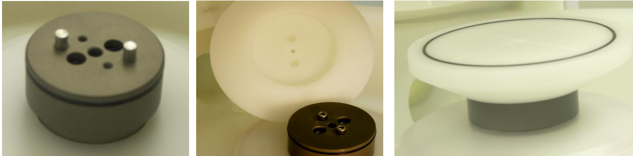
Figure 3-13 INSTALLING PRESS-ON CHUCK
