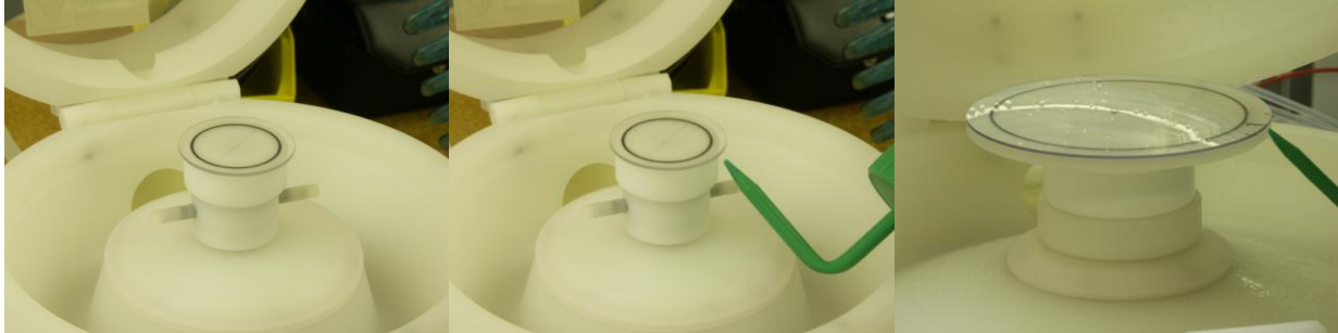
Figure 4-2 Wet Testing 1.75" and 200mm Chuck
