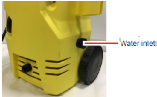
Figure 17 Pump water inlet
