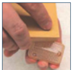
Sanding with micro-mesh sandpaper
