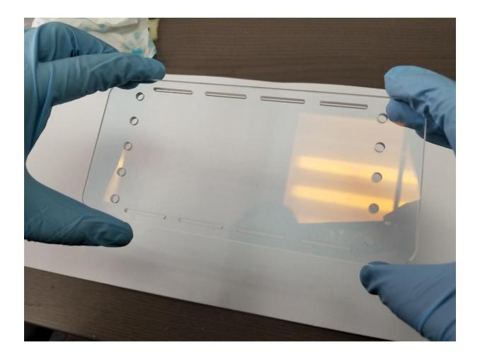
To inspect the UV Glass Filter., hold the glass filter from the edges. Once removed, look for any smudges, in bright light. If you see smudges, wash the UV glass using hot water and liquid soap. Dry using lint free cloth and compressed air. The UV Glass must be free from smudges and lint prior to installation
