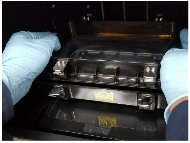
When putting in the VAT make sure **FRONT** is facing towards you, when installing.
