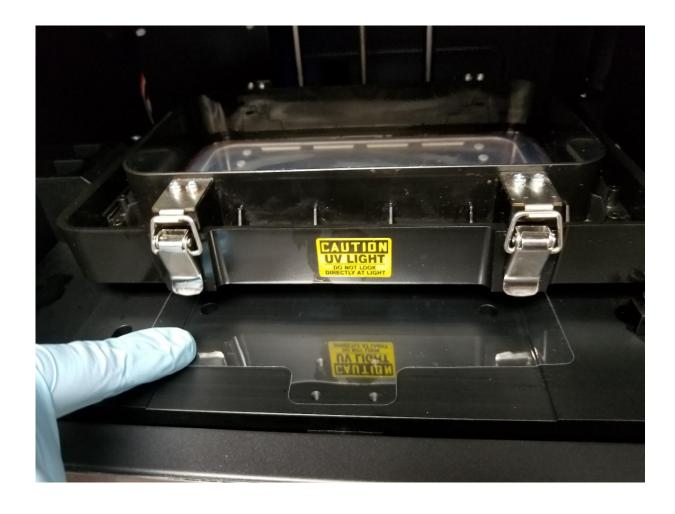
Keep the plastic under the foam intact. Do not remove or peel the piece of plastic.
