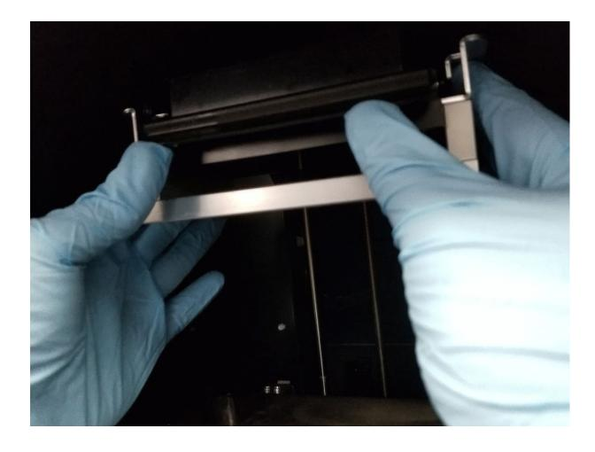
To Pull out the Built plate make sure to push handle to the high position. Lift at the front with both hands and slide out.
