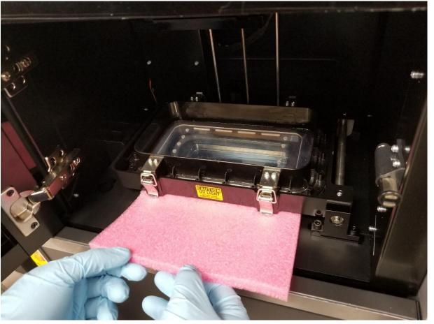
A protective foam support may be left in the machine for shipping purposes. Start by removing the foam.
