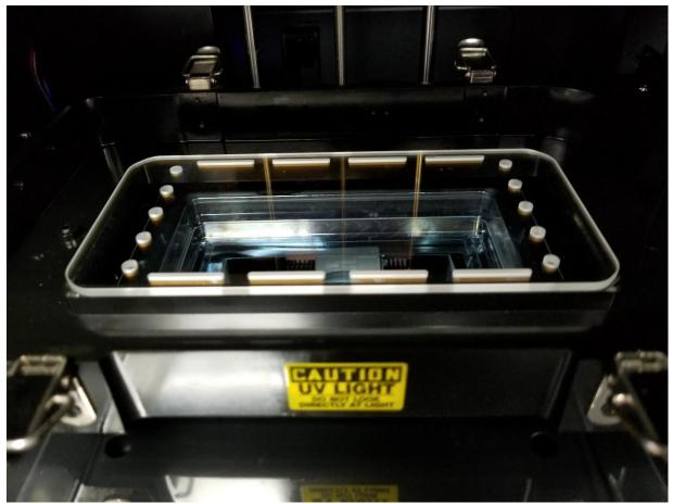
Once finished, place the UV glass between the four placement tabs.
