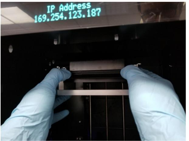
Make sure it is firmly in and push the handle down with both hands to secure the built plate.
