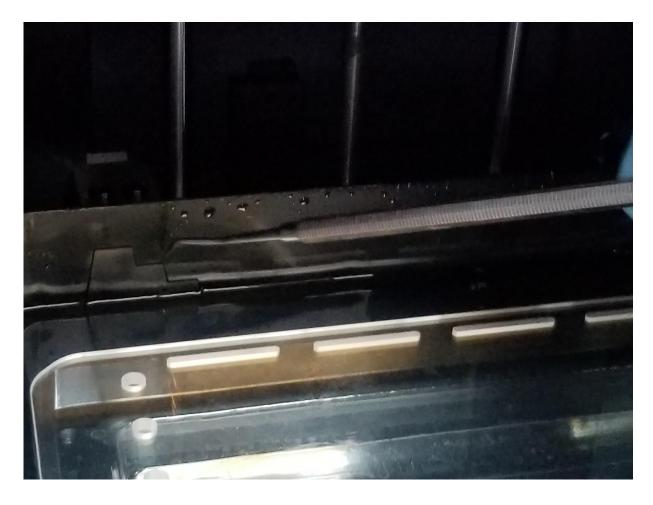
There is a level indicator located at the rear left side of the VAT. Maximum amount of resin should be not exceed the middle step.
