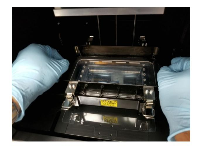
To remove the VAT use both hands and hold either side of the rim and lift the VAT upwards.
