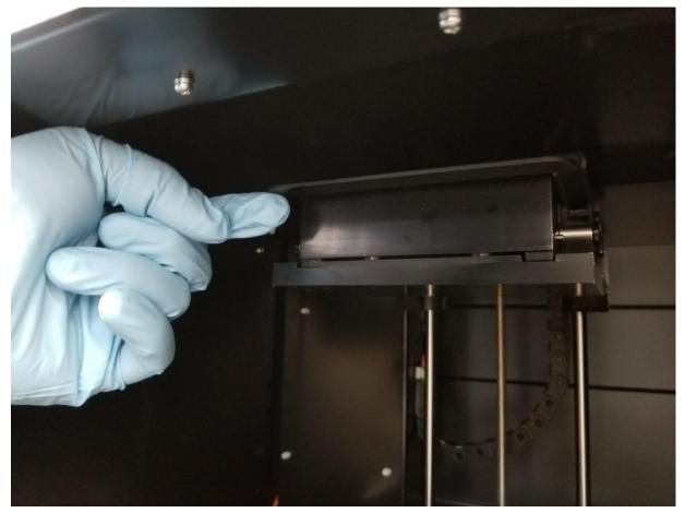
To install the built plate. Make sure the handle is in the high position.
