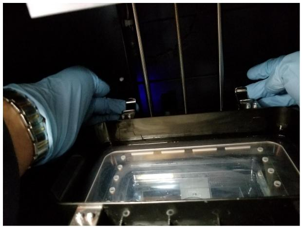
To remove the vat, start by unclipping the back clips.
