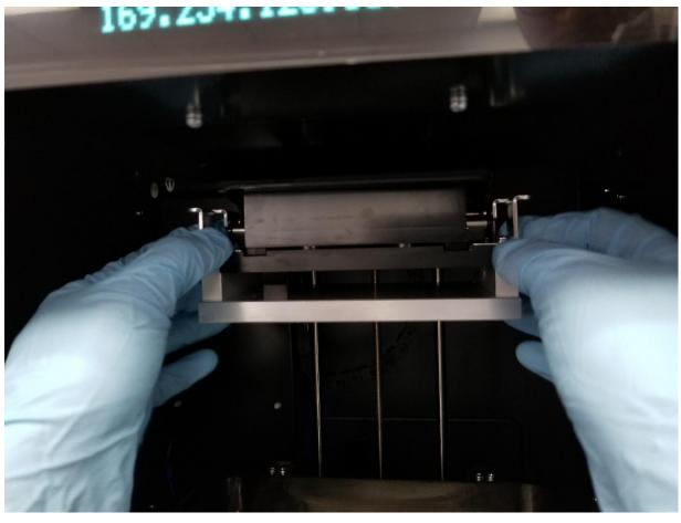
Slide the metal build plate tabs in the build assembly.
