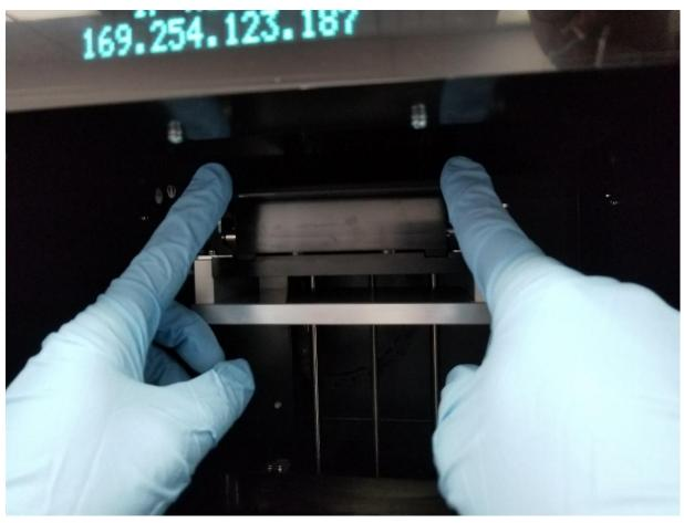
The build plate should slide all the way and drop.
