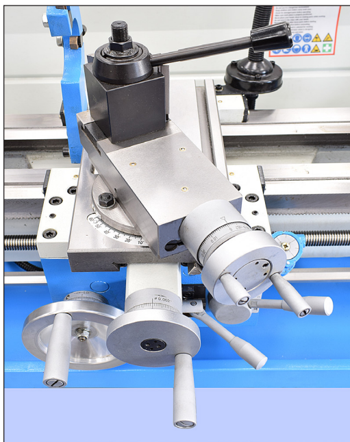
Figure 3-13 Cross-slide and compound dials Both collars are friction-coupled to their leadscrews by leaf springs. To zero a dial, or set it to any desired number, hold the handwheel firmly, then rotate the knurled rim.
