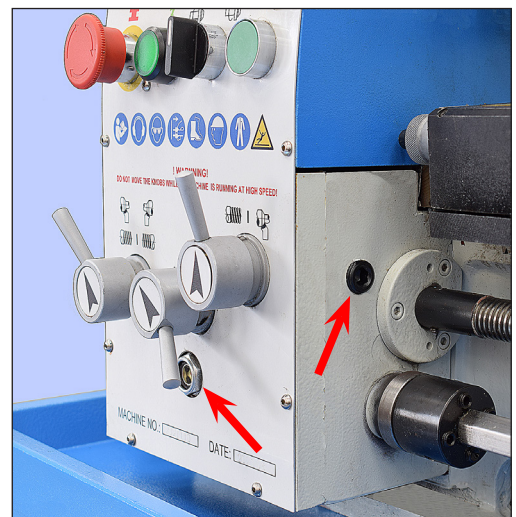
Figure 4-2 Gearbox sight glass & fill plug
