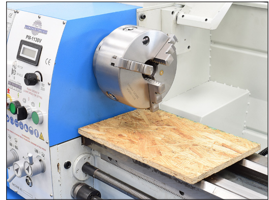
Figure 3-7 Protect the bed when removing or replacing a chuck. Chucks, faceplates and wrenches can seriously damage the bed if dropped.
