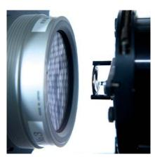
Inspecting surface roughness with an interferometer
