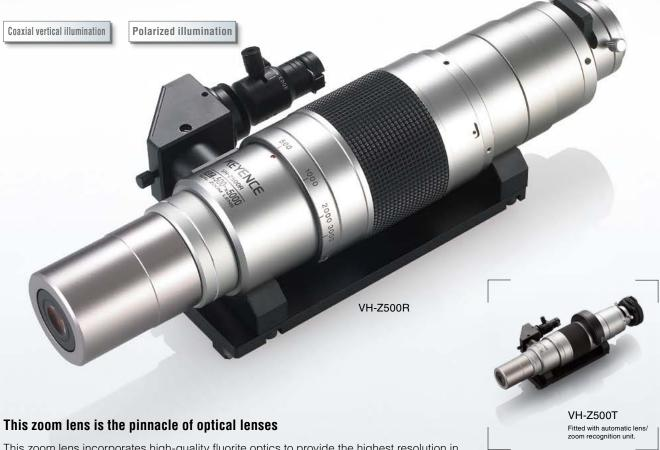
This zoom lens incorporates high-quality fluorite optics to provide the highest resolution in its class. The advanced 3D display function precisely reproduces images.
