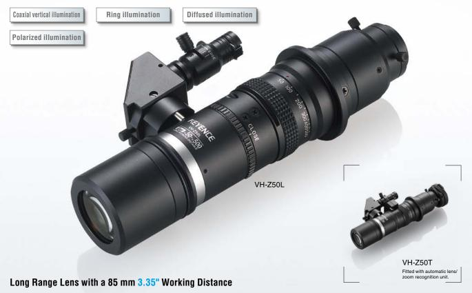
This lens uses cutting-edge optical design and advanced illumination technology to maintain an 85 mm 3.35" observation distance even at the maximum 500x magnification. It can capture recesses in the target clearly and it offers ample working space for dramatically improved observation efficiency.
