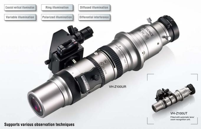
The VH-Z100UR inherits the optical design of the VH-Z100R, which offers a 25 mm 0.98" observation distance over the 100-1000x zoom range. It supports high-resolution observation in bright-field and dark-field over a wide zoom range, and can be used in various applications including polarization and differential interference observation.
