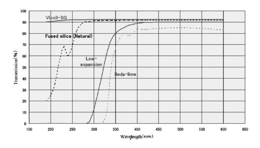
Optical transmission of synthetic quartz – Viosil-SQ (3200130 – 3200133)
