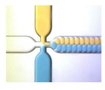
This image shows two aqueous droplet streams being generated simultaneously with a surfactant to prevent coalescence
