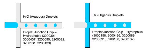
The hydrophobic coating is resistant to organic solvents. It can be removed using acidic or basic solutions, for example a 0.1M Sodium Hydroxide for 24 hours.
