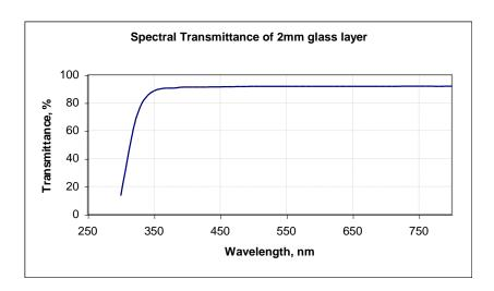
Optical transmission of glass (standard material)
