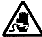
Caution, electrical shock
