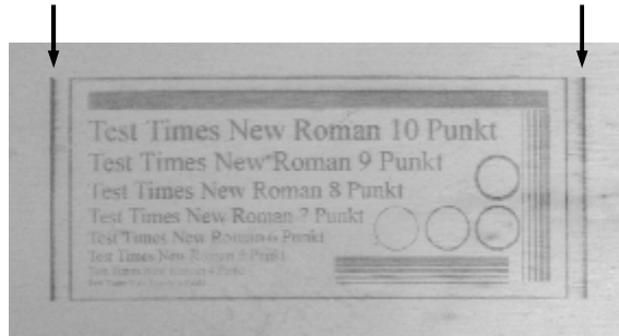
shadows beside the engraving, caused by too high tickle power
