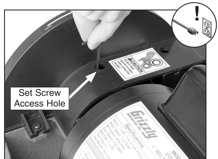
Figure 33. Location of access hole for the sanding disc set screw.
