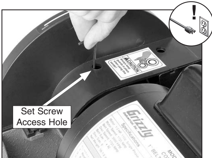
Figure 13. Securing the sanding disc set screw.
