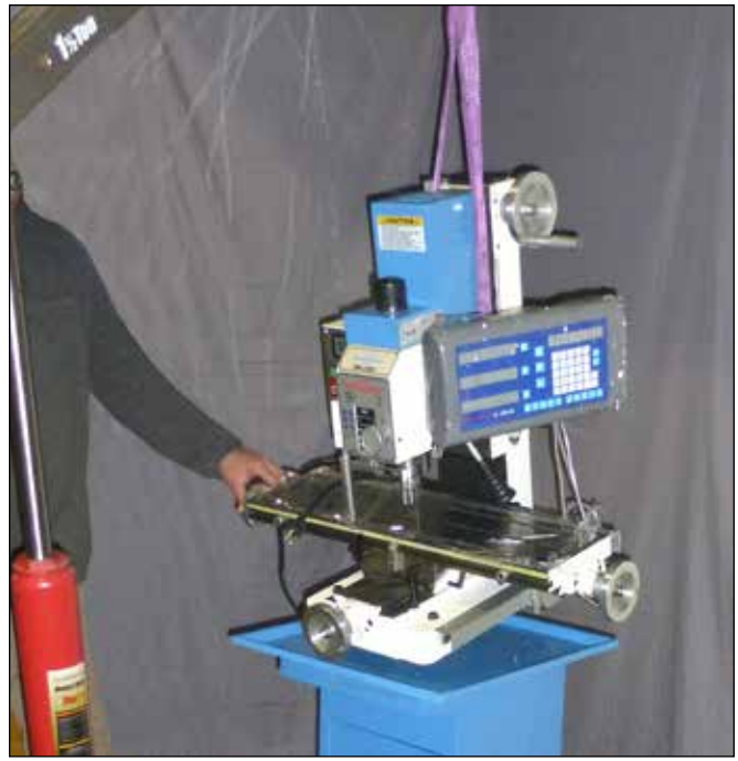
Figure 1-3 Lowering the mill into position
