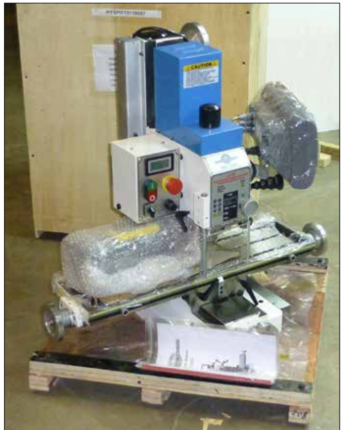
Figure 1-1 Mill ready for lifting
