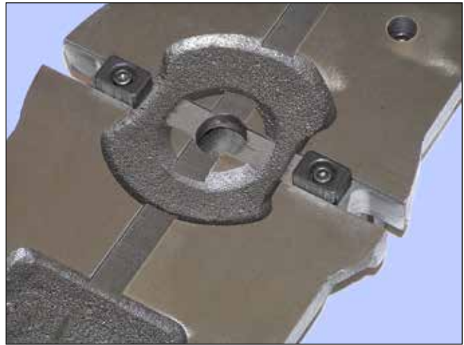
Figure 3-14 Vise keys installed on X-axis On most vises the keys can also be installed on the long axis.
