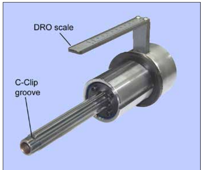
Figure 4-7 Complete DRO scale and quill assembly For illustration only: for servicing operations the scale should be detached from the quill and should remain in the DRO case.
