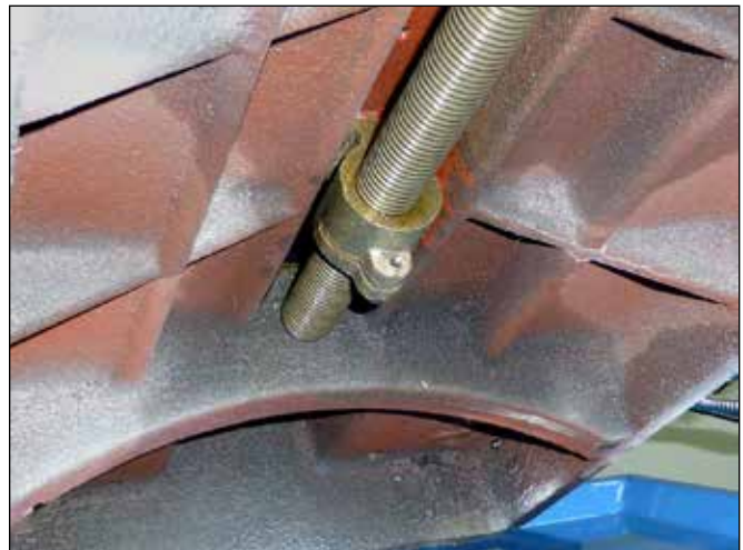
Figure 4-4 Y-axis backlash adjustment
