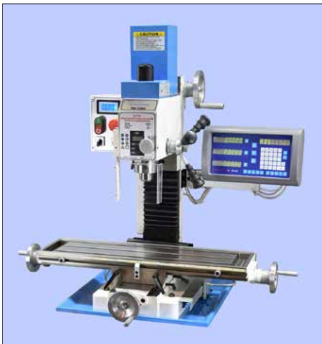
PM 25MV-BD with optional 3-axis DRO
