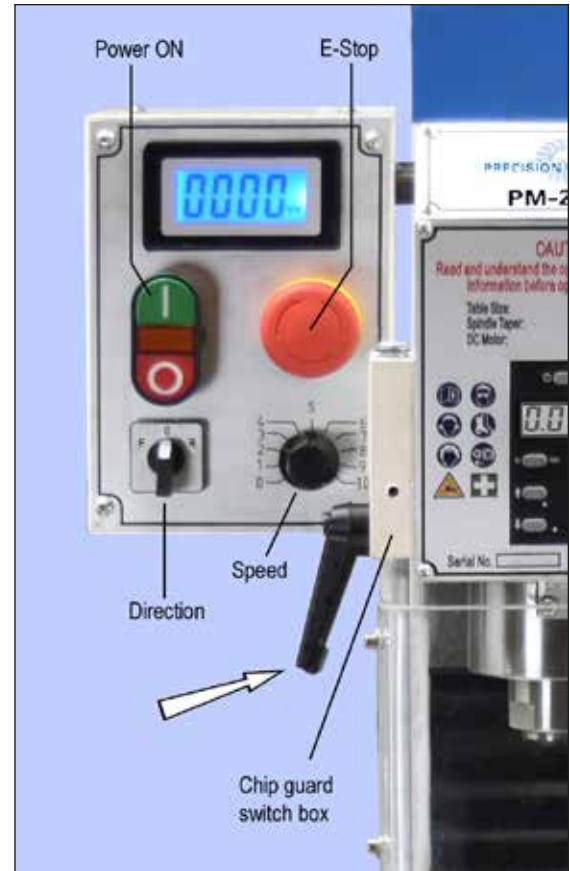
Figure 3-1 Spindle motor controls Also shown, arrowed, is the quill locking lever
