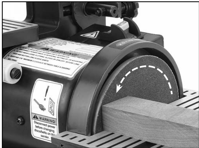
Figure 26. Disc rotation and workpiece position.
