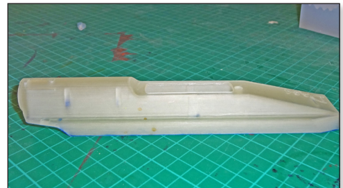
Figure 22: PolyJet pattern without optional sanding or priming is suitable for many silicone molding projects.
