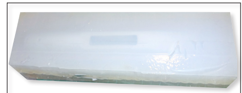
Figure 36: Pattern within the cured silicone mold.
