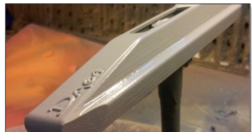
Figure 24: Primed patterns highlight areas that need additional finishing, if any.
