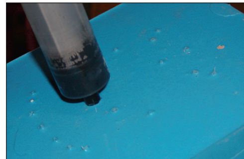
Figure 3: Casting urethane material (injection shown).
