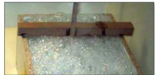
Figure 35: Place filled mold box in a vacuum chamber to remove air (degassing).
