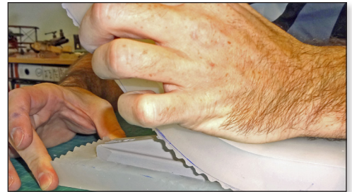
Figure 45: After curing, extract cast part from silicone mold.
