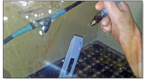
Figure 20: Use the Waterjet Station to remove support material.
