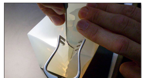
Figure 38: While cutting, pry the silicone material to open the cut.
