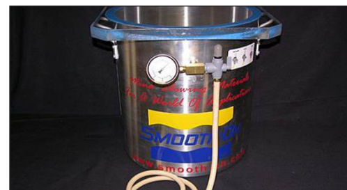
Figure 42: After pouring, place the mold in a vacuum chamber (shown) or pressure pot to remove air bubbles.
