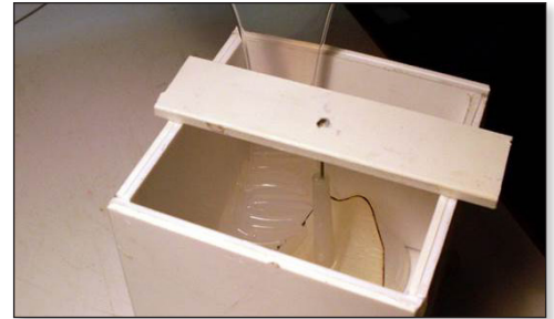
Figure 27: Use clear silicone so that the pattern is visible after mold curing.
