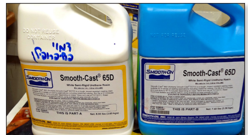
Figure 41: Weigh, mix and degas the cast urethane material.
