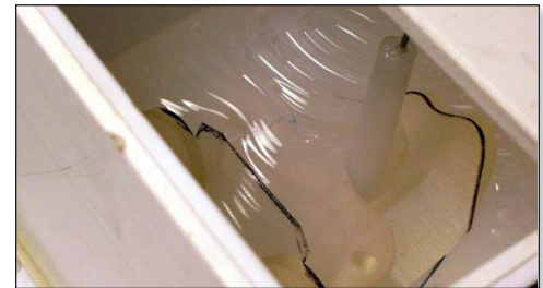
Figure 34: Slowly pour silicone into a corner of the mold box to avoid air pockets.
