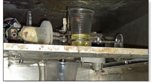
Figure 44: Inside a vacuum casting system: mold with fill funnel (bottom) and unmixed urethane (black liquid in center and yellow liquid above).
