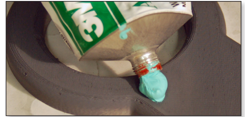
Figure 25: For high-gloss or clear castings, fill surface imperfections with spot putty.
