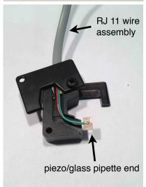
If you are able to obtain a good calibration scan from the new assembly and it can perform the "find surface routine" then it is functioning correctly.
