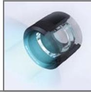
The variable illumination adapter is attached to the end of the lens and has a ring that, when turned, changes the incident angle of light from vertical to flanking illumination (approx. 10 degrees). This allows easier observation of minute height differences or scratches.
