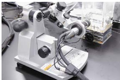
Stent fatigue test setup
