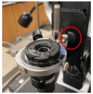
5) Lift the objective straight up off the mounting post on the microscope body and place carefully in the drawer located under the Keyence computer.
