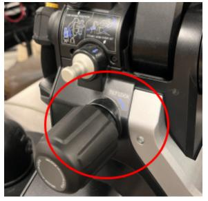
2) With a HAND ON THE MICROSCOPE HEAD rotate the locking lever counter clockwise to its vertical position
