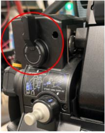
3) Tilt the head to its desired angle using the handles on the microscope body
