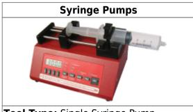
**Tool Type:** Single Syringe Pump **Location:** Microfluidics Lab - Elings 3430
