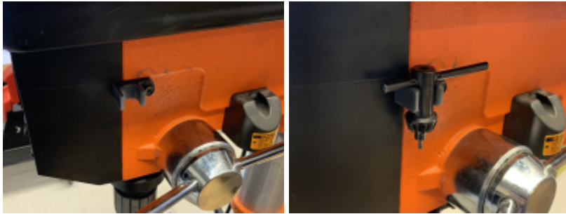
Printed replacement cabinet door latch
