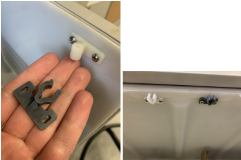
Printed replacement cabinet door latch
