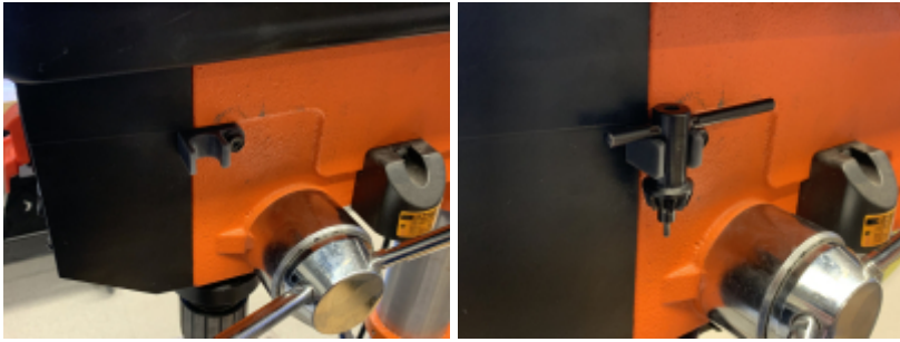
Printed replacement cabinet door latch
