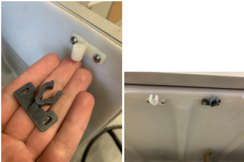
Printed replacement cabinet door latch
