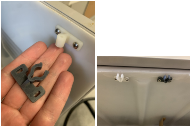
Printed replacement cabinet door latch
