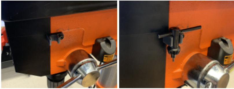
Printed replacement cabinet door latch
