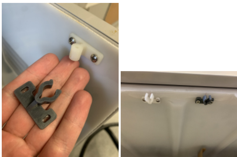
Printed replacement cabinet door latch
