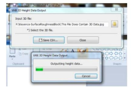
The exported .csv files contain height data in microns. No x and y data is given, for these you should refer to the datasheet on 3D pixel sizes.
