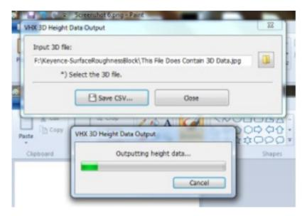
The exported .csv files contain height data in microns. No x and y data is given, for these you should refer to the datasheet on 3D pixel sizes.
