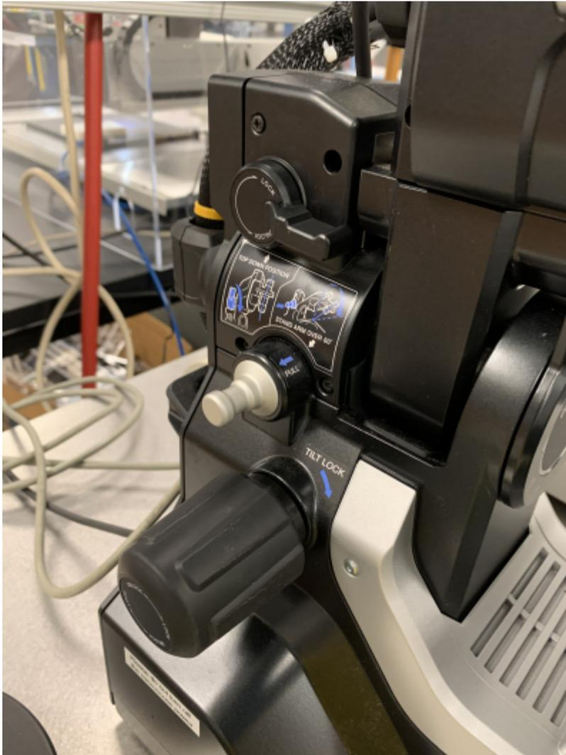
1. Loosen the tilt lock knob a turn or two max (until the knob loosens)
