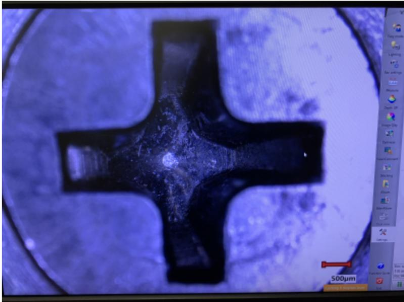
3. Click “3D Display” on the Keyence control pad and the microscope will scan up the object and create a 3D file which can be analyzed for depth.
