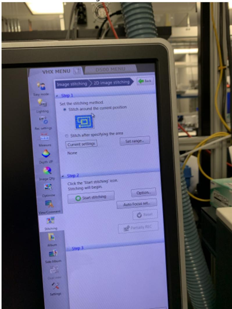
1. Center the sample in the frame and select "stitching" from the sidebar
