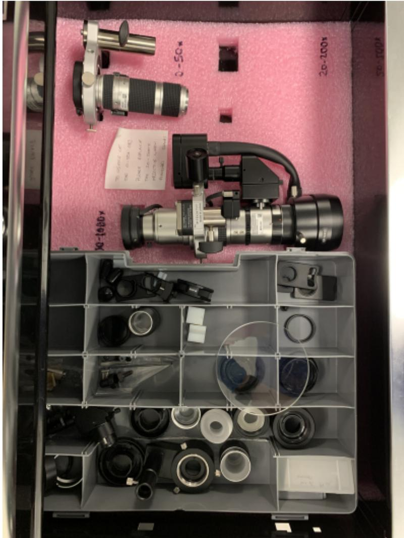
1. Switching to fiberoptic Epi-illumination for 100-1000x objective
