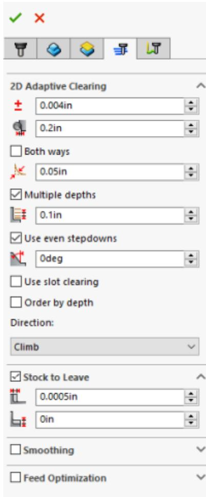
1. Part of feeds and speeds, HSM Works will auto fill many of the boxes, however due to the limited power and rigidity of the machine, stepdowns should be reduced based on the reference material and “multiple passes” should be used to reduce cutter load
