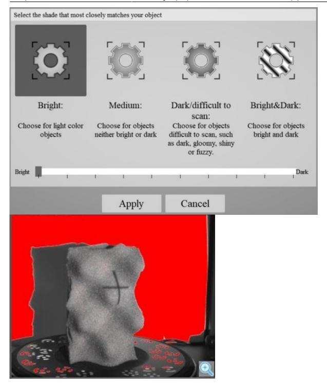
• Once a texture mode is selected, the brightness slider will appear. Use the camera screen in the upper right as a reference for adjusting the brightness level. Move the slider so that the crosshair is clearly illuminated on the object in the view window, but not so brightly illuminated that red areas show up on the object to be scanned. An example image of the right exposure over the part is shown.
