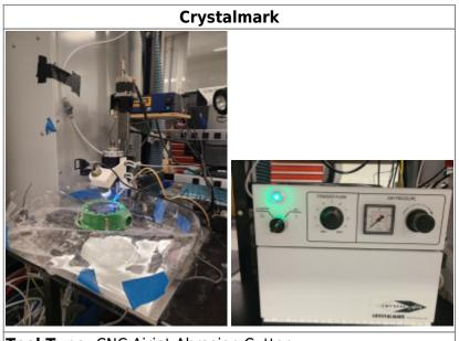
Tool Type: CNC Airjet Abrasion Cutter
