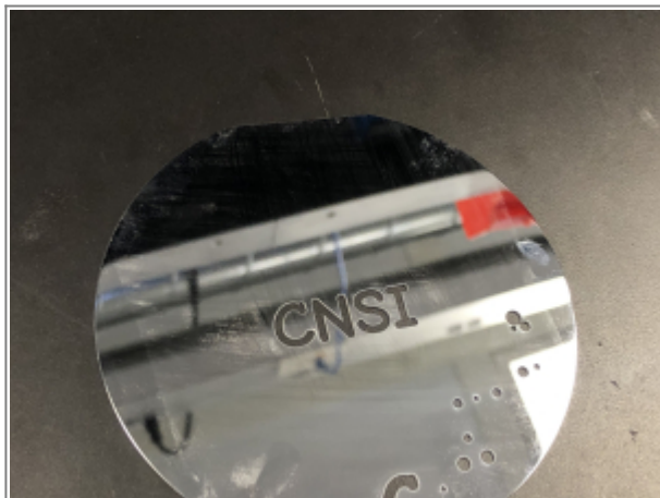
Contour cut in 0.5mm SI wafer
