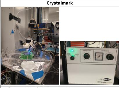
Tool Type: CNC Airjet Abrasion Cutter
