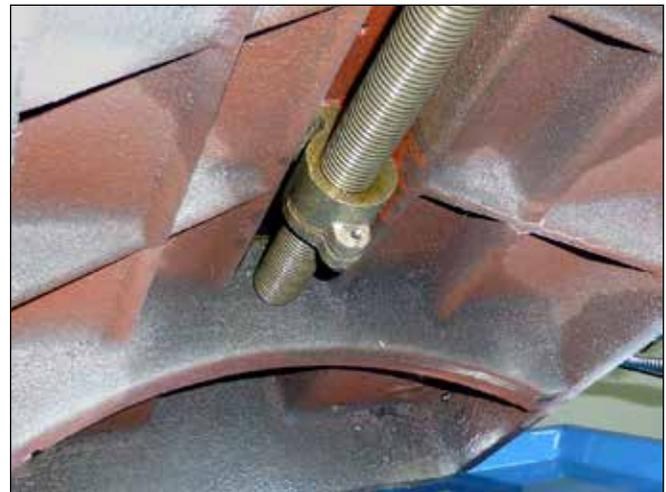
Figure 4-4 **Y-axis backlash adjustment**
