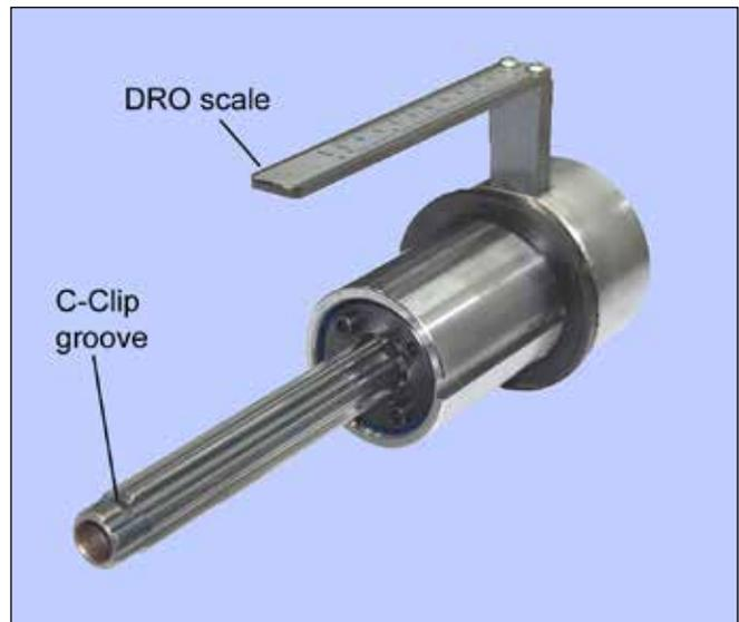
Figure 4-7 Complete DRO scale and quill assembly
